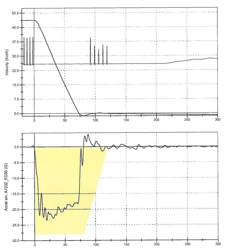
Continuous time under -15.0 G was 61.0 ms Total time under -20.0 G was 30.7 ms Sled Decel Peak = -23.5 G Sled Plateau Average Level = -20.6 G Sled Pulse Duration = 80.9 ms
